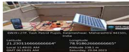
Fig 6: Testing of P&O MPPT with different tilt angle and weather conditions
