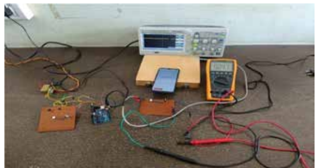
Fig 4: Hardware test of single phase automatic soft starter prototype
